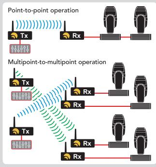
W-DMX is unique in its use of certain advanced radio techniques which are more often found in mobile phone and military communications. Rather than using fixed frequency channels, W-DMX uses adaptive frequency hopping technology (as well as TDMA and GFSK technoliues) to continually check for interference and to rapidly move operation over to clear radio channels. The frequency hops occur one thousand times every second to ensure smooth, efficient and robust operation.
