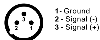
DMX-OUT XLR Connector - Socket:
