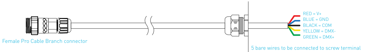
5 bare wires to be connected to screw terminal
