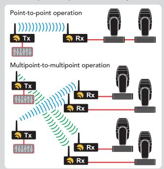
W-DMX<sup>™</sup> is unique in its use of certain advanced radio techniques which are more often found in mobile phone and military communications. Rather than using fixed frequency channels, W-DMX<sup>™</sup> uses adaptive frequency hopping technology (as well as TDMA and GFSK techniques) to continually check for interference and to rapidly move operation over to clear radio channels. The frequency hops occur one thousand times every second to ensure smooth, efficient and robust operation.
