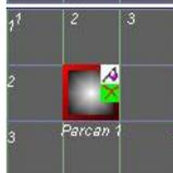
This flag is displayed when a fixture is excluded from an effect. Fixtures marked with this flag are masked from the parameter effect.
