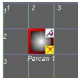
This flag is displayed when a fixture is excluded from a chase. Fixtures marked with this flag are masked from the parameter chase.
