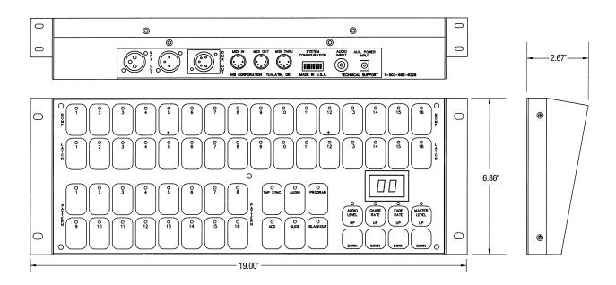
The TLC 16 lighting and effect console provides a variety of control options in a touch panel format.
