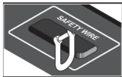
Fasten a safety cable (not shown) between the support structure and the attachment point on the device. The safety cable must be able to bear at least 10 times the weight of the device.
