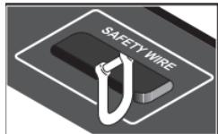
Fasten a safety cable (not shown) between the support structure and the attachment point on the device. The safety cable must be able to bear at least 10 times the weight of the device.
