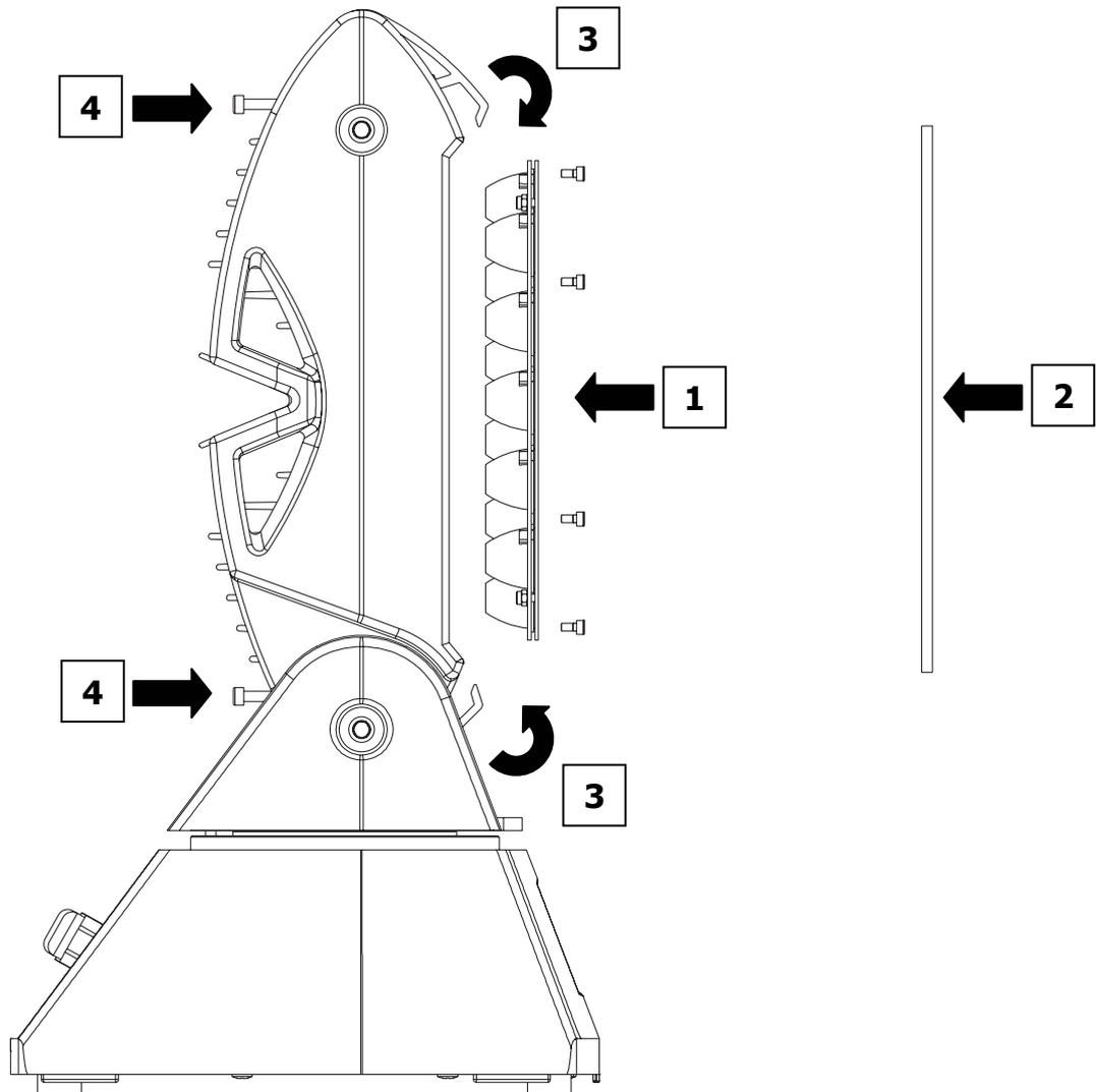
**1** Carefully position the new set of lenses, paying particular attention to the alignment of the LEDs in relation to the lenses.
