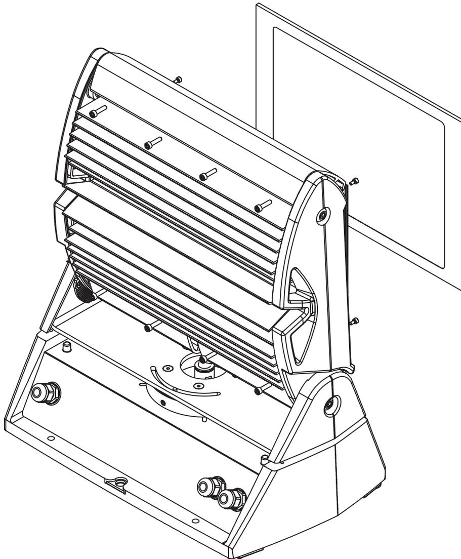
Rotating the two shells toward the front of the fixture, the front glass can be removed for access to the lens-holder panel.
