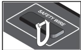
Fasten a safety cable (not shown) between the support structure and the attachment point on the device. The safety cable must be approved for a safe working load (SWL) of 10 times the weight of the device.
