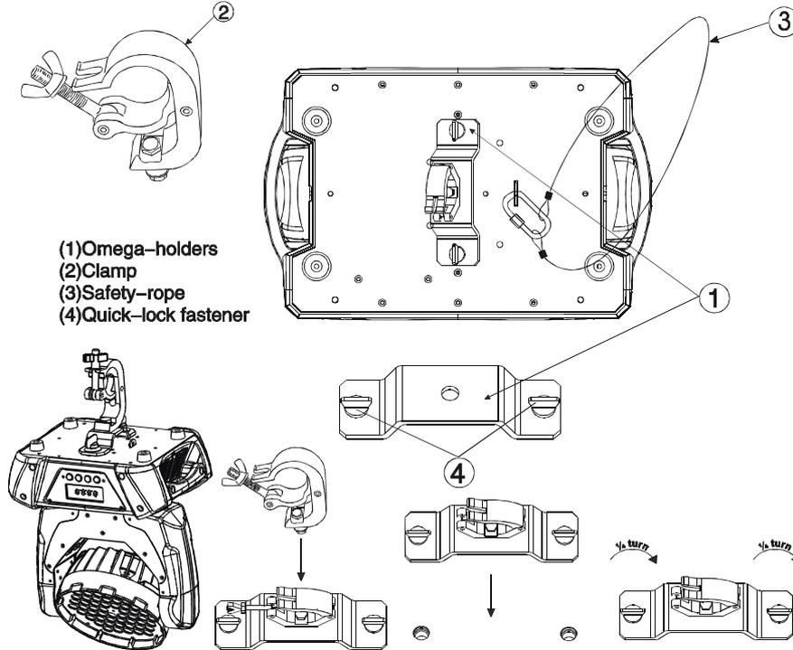
Screw one clamp each via a M12 screw and nut onto the Omega holders. Insert the quick-lock fasteners of the first Omega holder into the respective holes on the bottom of the device. Tighten the quick-lock fasteners fully clockwise. Install the second Omega holder. Pull the safety-rope through the holes on the bottom of the base and over the trussing system or a safe fixation spot. Insert the end in the carabine and tighten the safety screw.
