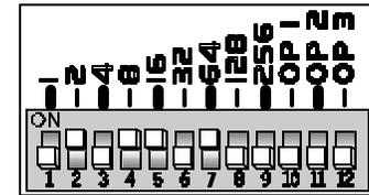
Addressing multiple fixtures of the same type is accomplished by simply adding the number of channels required to the start address of the first fixture to yield the start address of the next fixture.
