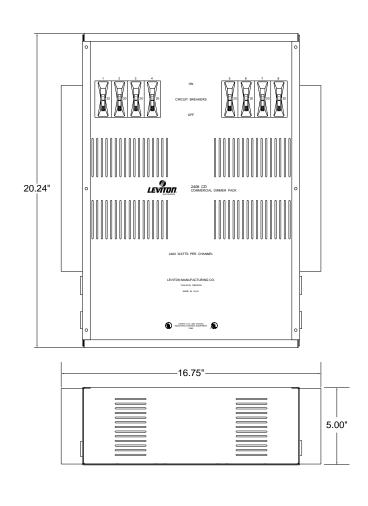
These UL listed commercial dimmer packs feature input ports for all the communication protocols you'll need, including NSI's Micro-Plex, DMX512, NSI Luma-Net® and 0-10V analog. The 2408 also features epoxy encased toroidal filters, which minimize noise and have a rise time of 400 micro-seconds. Combine with Luma-Net control stations or any Leviton-NSI control console for a totally integrated lighting system.
