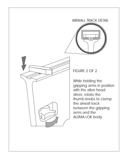
By "thumbing" the thumb knobs clockwise you have clamped the ALUMA-LOK to the airwall track.
