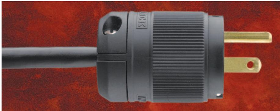
*Because of its unique design, a Clamp-Lock termination actually tightens when the cable is pulled. This eliminates terminal self-loosening due to heat, shock or vibration.*
