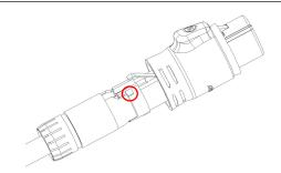
(6) After the assembly of the cable clamp, inner core and housing, tighten the boot in a clockwise direction.
