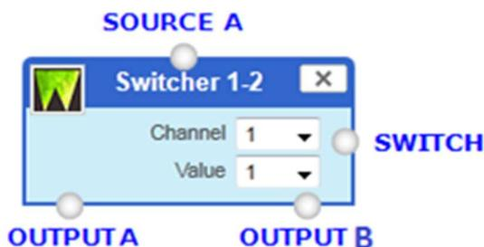
**Switcher 1-2:** Controllable Switch operator, when the trigger channel (Switch) is greater than the set value, OUTPUT B is output, in other cases OUTPUT A is output. Must have all input sources and output sources connected
