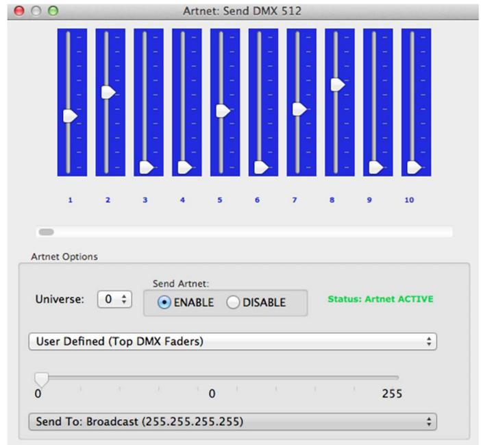
When first opened, the Art-Net is set to Disabled, please set it to Enabled, and then you can use either the DMX faders to test one or more DMX channels, or use the test-patterns from the options available.
