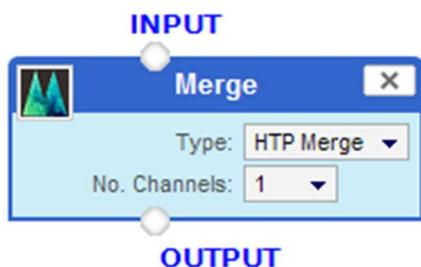
**Merge:** HTP or LTP merge operator, drag as many lines to the input node as you wish to merge
