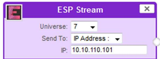
ESP Stream: ENTTEC Show protocol DMX over Ethernet stream (ESP). IP address is the destination address used when the stream is sending data only.
