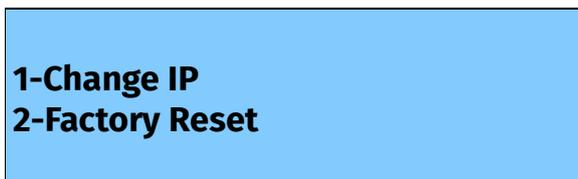
Setup screen allows changing the IP address of the unit via "Change IP" or doing Factory Reset.
