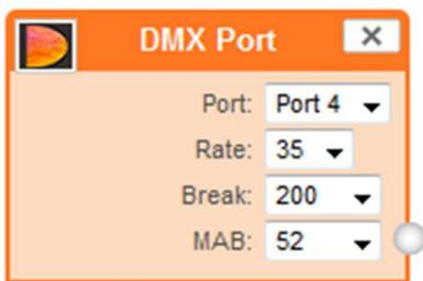
The DMX port represents one of the physical ports on the rear of this unit, select which port you want to use by using the drop down.
