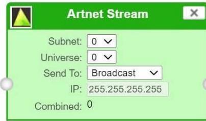
Art-Net Stream: "Send IP address": is the destination address used when the stream is sending data only (Unicast).
