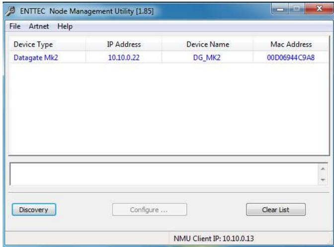
NMU (Node Management Utility) is a free Windows and OSX application that is used to manage compatible ENTTEC DMX over Ethernet nodes. NMU will not directly allow you to configure the Datagate Mk2 itself, but it can help you find your unit's IP address and then open a browser window to make the required changes.
