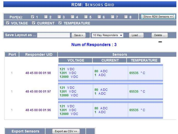
RDM Sensors page, allows discovering all RDM devices and monitoring all sensors supported by RDM tool. Examples include: Temperature, Current and, Voltage sensors.
