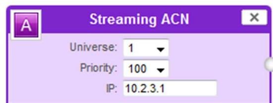
Streaming ACN: "IP address" is the destination address used when the stream is sending data only (default is disabled = 0.0.0.0)
