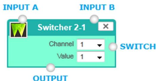
**Switcher 2-1:** Controllable Switch operator, acts as a normal Input A to Output Action, but when the trigger
