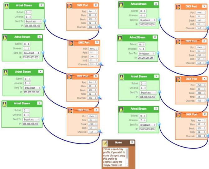
Create a new profile or edit an existing one using the profile-editor. Opens up in a new page in your web browser. Select a module on the left and the right panel will provide help about that panel. Connect a module to another using wires from one point to another. The direction of the wire (arrow) is important, the arrow signifies output, and reflects the flow of data.
