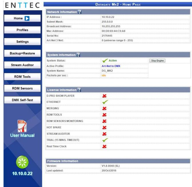
The Datagate Mk2 is configured, controlled and programmed through a web browser interface running on a computer system located on the same Local Area Network. Any modern web browser, such as Chrome, Firefox, Internet Explorer, Safari or Opera, running under any operating system, including Windows XP or Vista, Mac OS X or Linux can be used.
