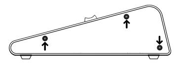
Attach the PIVOT WING 512 to the PIVOT CUE 512 left side using the supplied plate and four screws.
