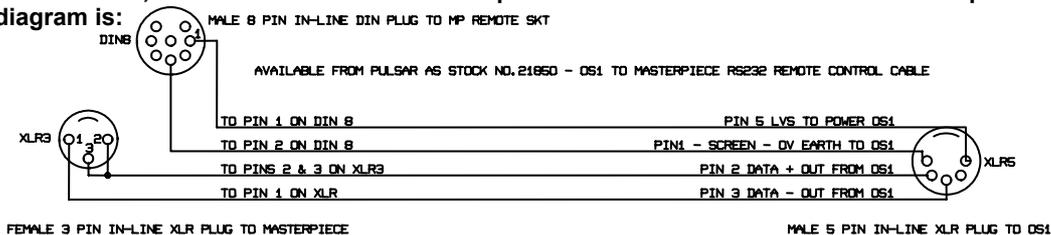
DIN SOCKET POWERS OS1. XLR3 CARRIES PMX (RS232) DATA TO REMOTELY CONTROL THE MASTERPIECE
