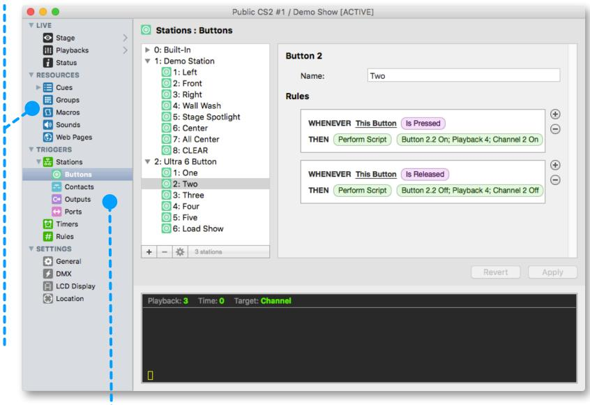
The Settings section is used to edit DMX resources, universe and playback settings, LCD Display and Location settings.
