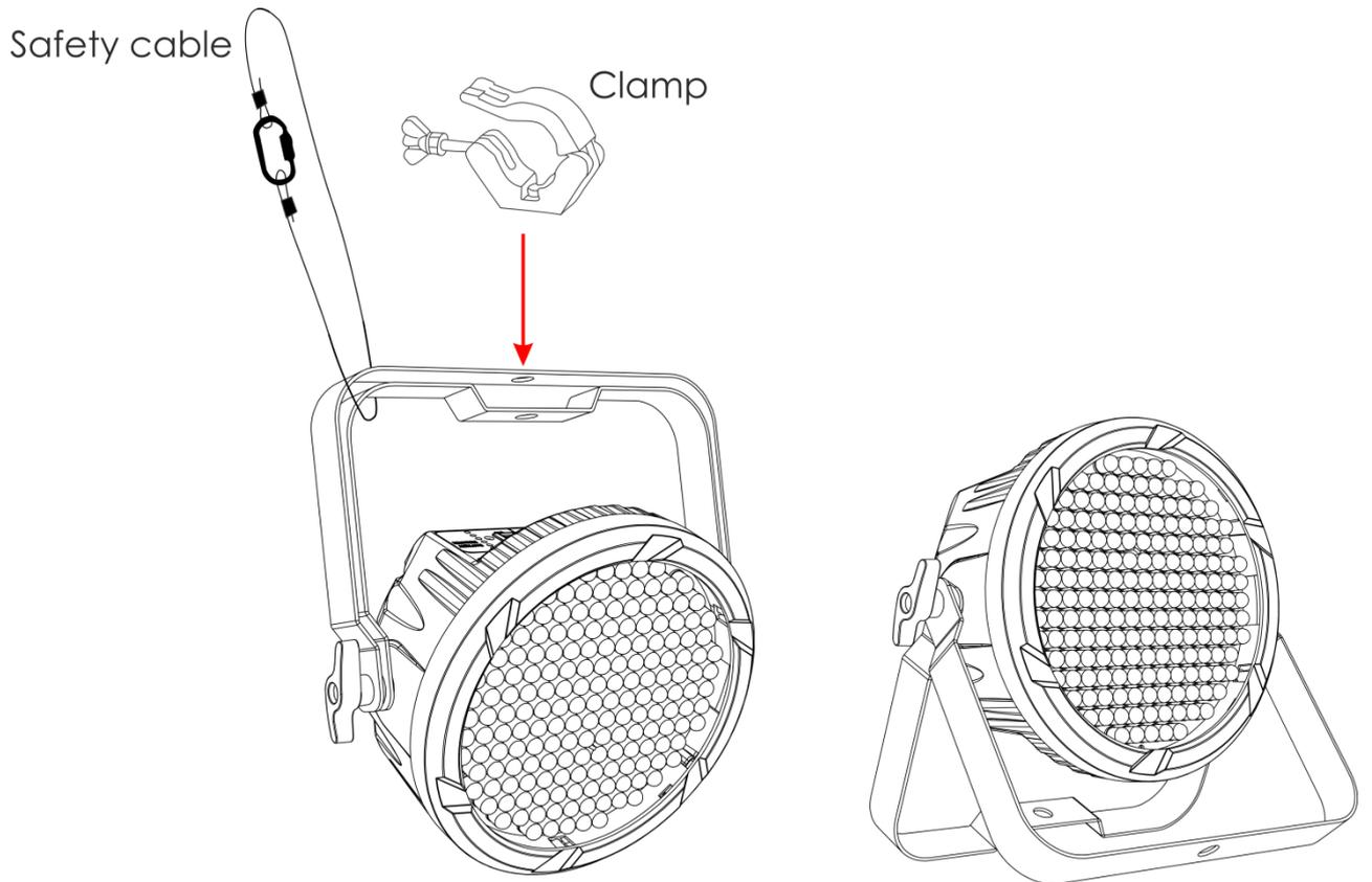
The EventLITE 177IR can be placed on a flat stage floor or mounted to any kind of truss with a clamp.
