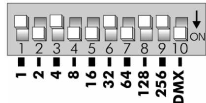
Addressing multiple fixtures of the same type is accomplished by simply adding the number of channels required to the start address of the first fixture to yield the start address of the next fixture. Although this fixture can be used in modes that occupy less than 12 channels, it is highly recommended that the units are still addressed 12 channels apart. This reduces the chances of data overlapping if the console or control is to become temporarily mis-configured or unstable.
