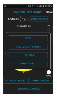
• **Reset** - selecting this will reset the fixture to its default factory settings. Do this if you are running into programming issues.
