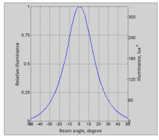
\* Illuminance is measured at a distance of 6.7m. For additional information refer to Lux diagram.
