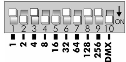
Addressing multiple fixtures of the same type is accomplished by simply adding the number of channels required to the start address of the first fixture to yield the start address of the next fixture. This fixture occupies **2** channels.
