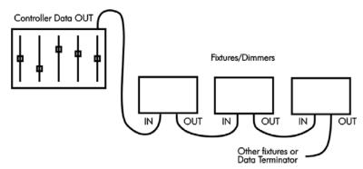
The DMX Standard calls for connections between DMX compatible equipment to be made using 5 pin XLR connectors. However, it is common to see fixtures with 3 pin XLR connectors as these types of balanced or "Lo-Z" cables are common in the audio industry. In either case, pin numbers are the same and carry the same signals.
