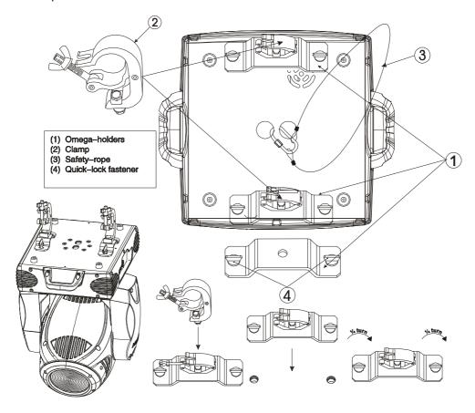
Screw one clamp each via a M12 screw and nut onto the Omega holders.
