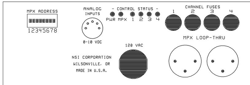
**ANALOG 0 - 10 VDC CONTROL WIRING.**
