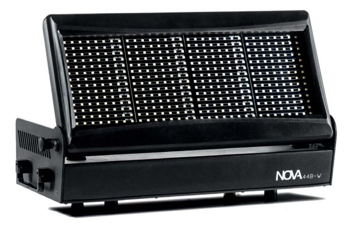
The Nova Strobe is a LED flood light and ambience blinder with a light output of 40.000 lumen, and can be controlled in 4 segments. The 446 white LEDs create a bright light in 6.500K colour temperature.
