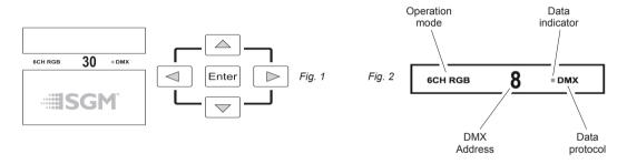
When the product is switched on, the fixture will be at its default setting showing the ROOT menu (Fig. 2).
