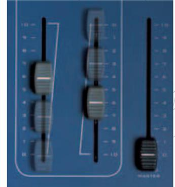
The motorized A and B Masters automatically follow crossfades between scene A and scene B, constantly showing overall output values.
