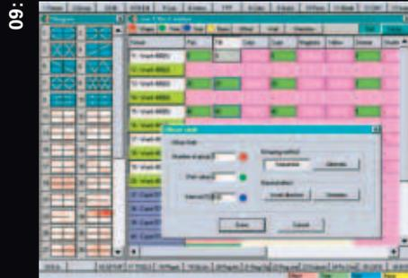
09: **REGIA 2048 OPERA, REGIA 2048 LIVE** and **REGIA 2048 PRO** are very versatile consoles, with a series of functions which enable operators to program a single effect or an entire show rapidly and efficiently, controlling up to 2048 DMX channels.
